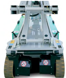
New design of the chassis allows easy cleaning and ensures protection to the components
