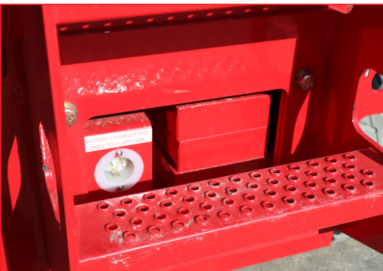
SINGLE PLUG FOR DECK POWER/CHARGER
